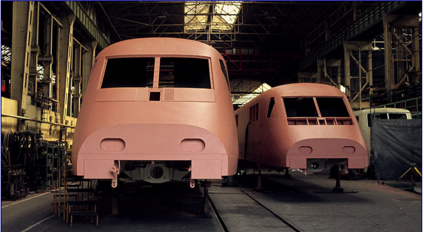
The vehicle bodies for the power cars were manufactured in the M3 workshop at Krupp in Essen. On 31 July 1984, both bodies had already been primed: 410 001-2 on the left and 410 002-0 on the right, which was transported to Henschel in Kassel for final assembly shortly afterwards. Photo: Ulrich Budde | Bundesbahnzeit
