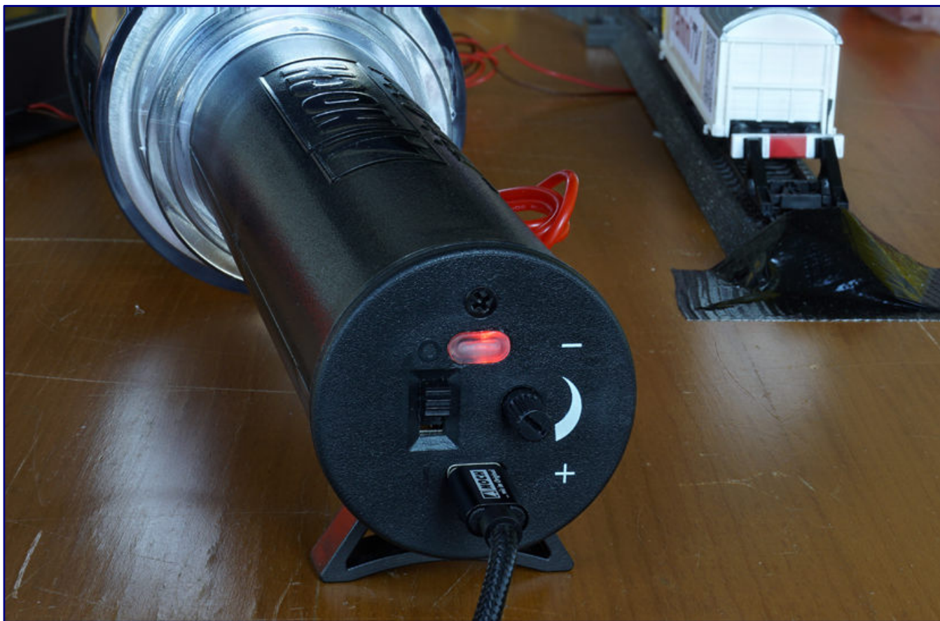
The fourth generation of the Gras-Master operates with an integrated Li-ion battery. A suitable "USB-A to USB-C" cable is included for charging. When plugged in and connected to a suitable power supply, a red LED indicates that charging is in progress.
