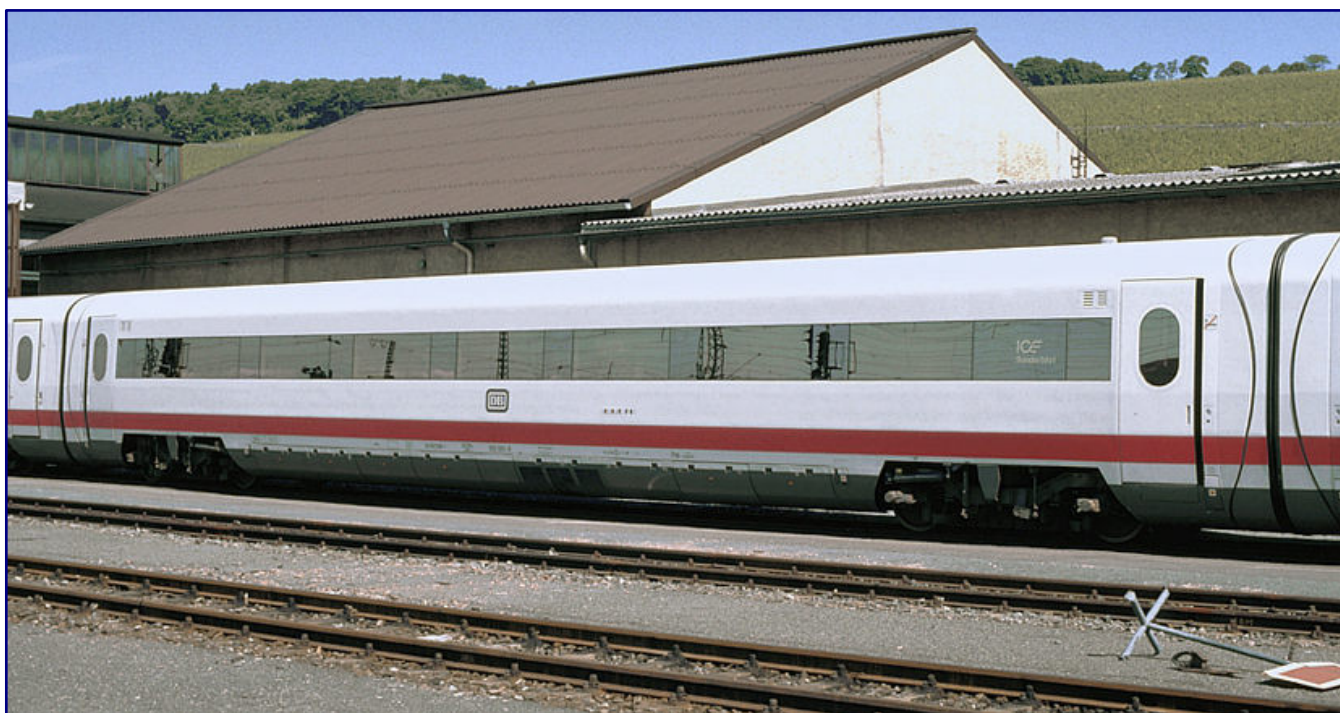
On 11 July 1988, 810 001-8 (demonstration car 1) in Würzburg offers a glimpse of its air-suspended MAN coupling frame bogies, which Märklin intends to reproduce with the Fiat bogies. Photo: Ulrich Budde | Bundesbahnzeit
