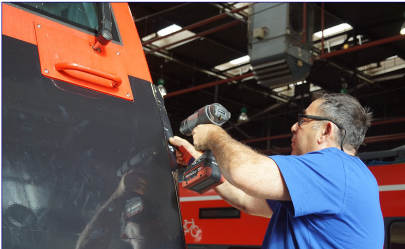
Decaling begins on the front of driver's cab 2. The first black foils have been applied, cut out at the grip plates and arrived at the transition to the bevelled edge. The hot air gun is needed here to apply and align along this edge.
