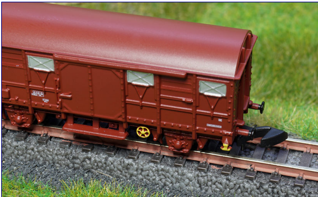
The UIC rope hooks have also been painted yellow on the new injection moulded overlays. The buffers have also been painted black.
