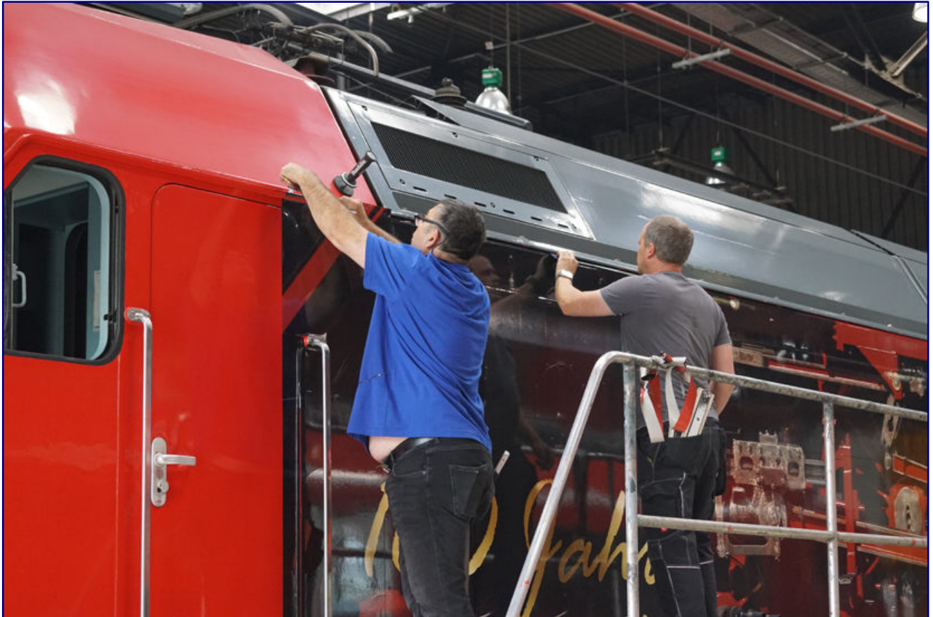
The fourth roll is being processed. In addition to the fan in the roof area, the picture also shows one of the bar magnets used to fix the adhesive films before removing the protective film in order to align them first.
