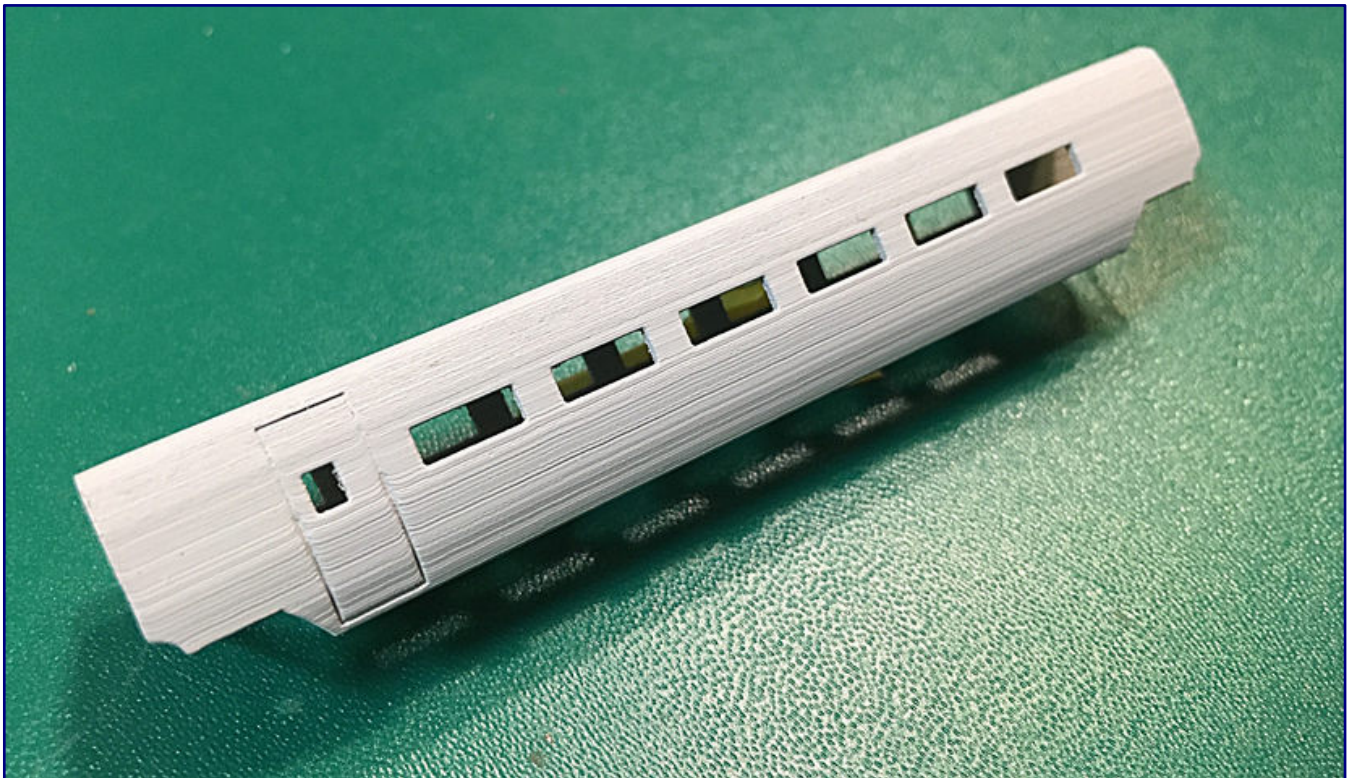
The light grey primed housing reveals the print layers and shows the need for reworking described in the text.
