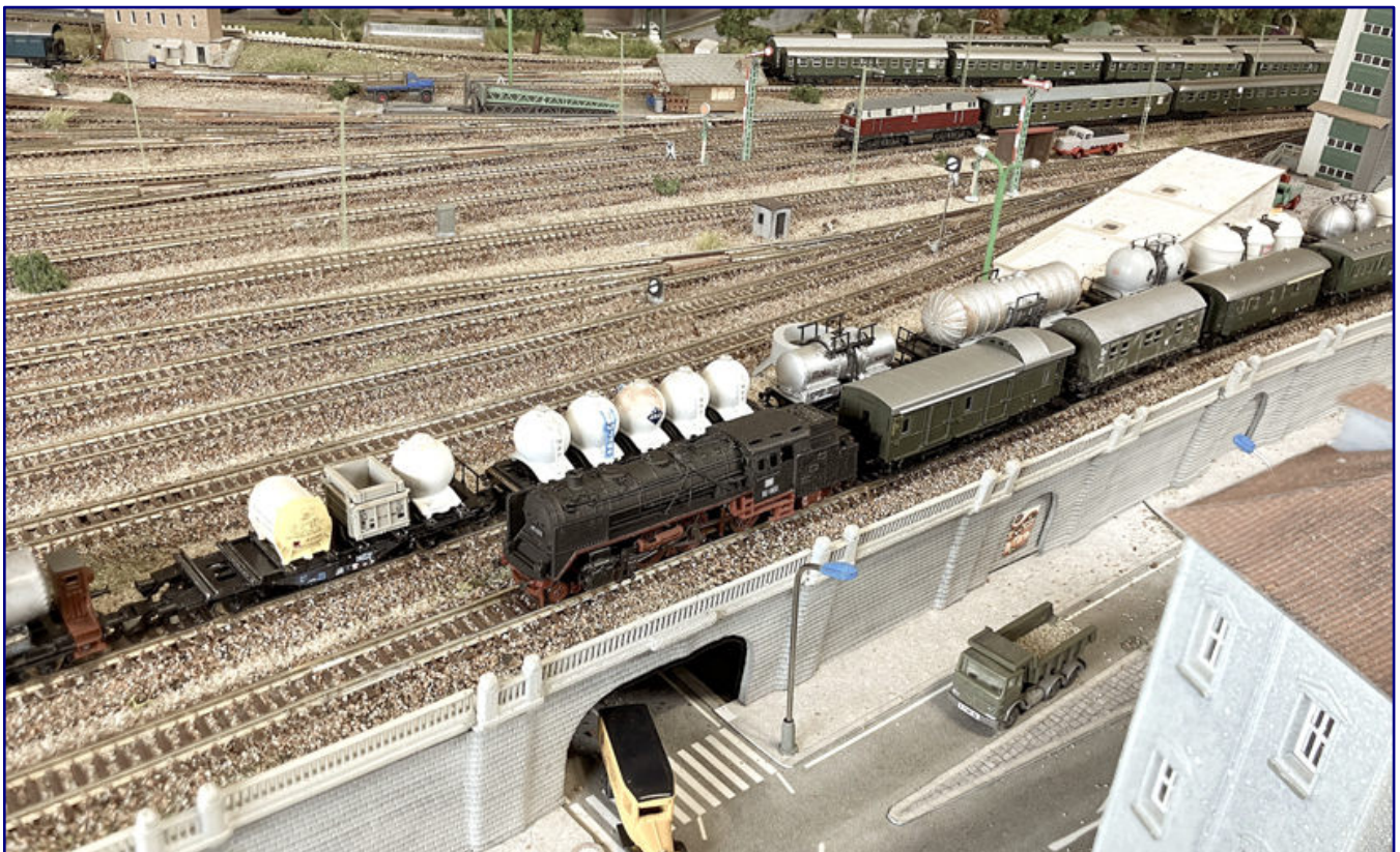
The Class 62 tank locomotive overtakes a freight train with its local passenger train. Its spherical door-to-door containers were also designed in-house and produced using 3D printing.
