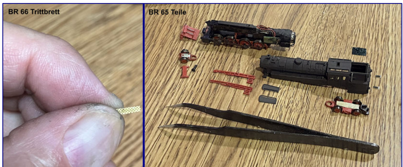
The 66 series requires a brass-etched bar, which is still to be painted red (left image). On the chassis of the 65 series (right image), the bell-type armature mount was ground down so that the housing could be fitted. The holder for the front wheel has been shortened and has no coupling; for the rear wheels, a new holder with a coupling shaft has been printed from resin.
