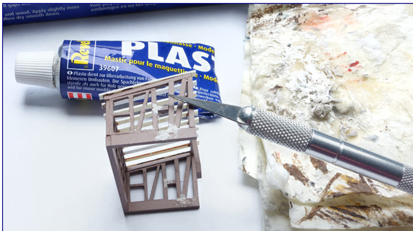
Joints and gaps that affect the appearance are filled with Revell modelling filler, sanded, and painted over again.
