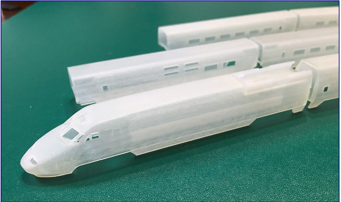
This is what the printed blanks looked like when they arrived from Shapeways. Mould changes were still required on the power cars to turn the TGV Atlantique into its predecessor, the TGV PSE.
