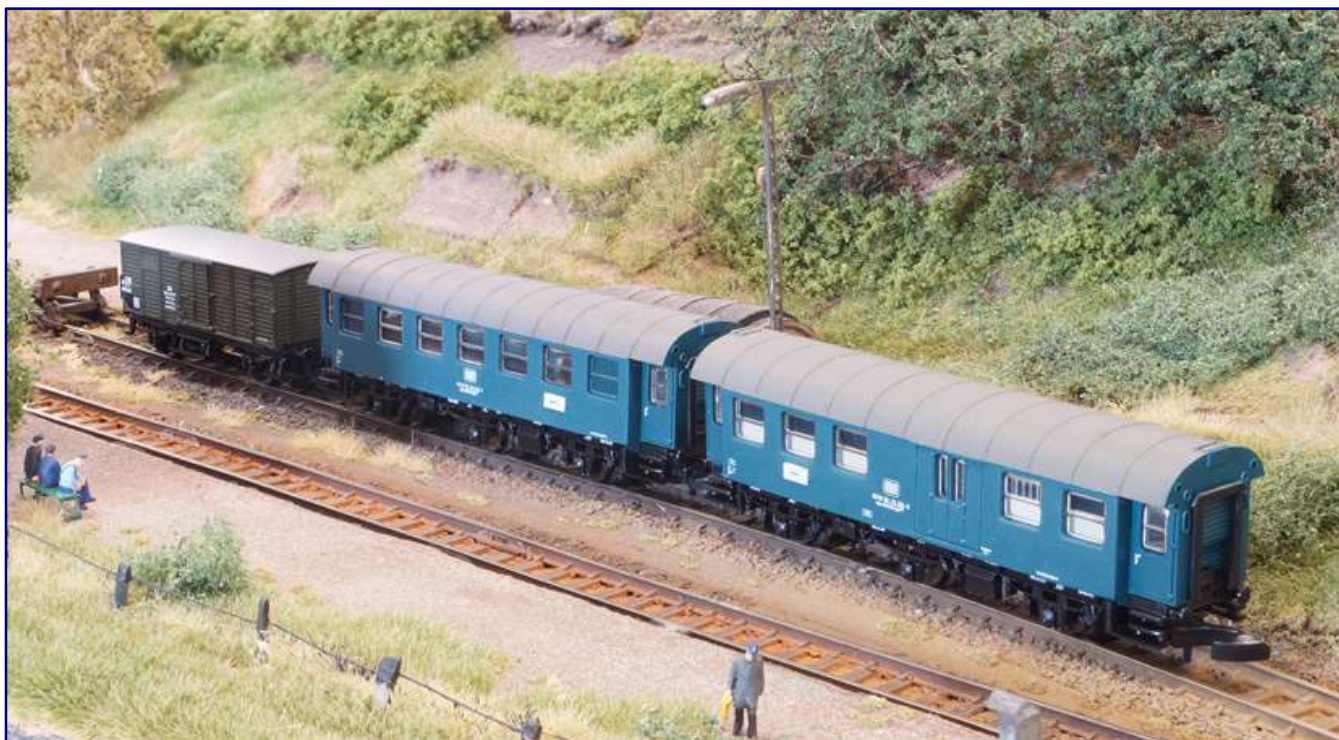
Railroad maintenance car trains often lined up at loading roads and were parked there for long periods during maintenance work. This was especially true for material, recreation, sleeping, and workshop cars. This offers attractive possibilities for model railways, as shown here with the workers taking a break and the brake shoe applier.
