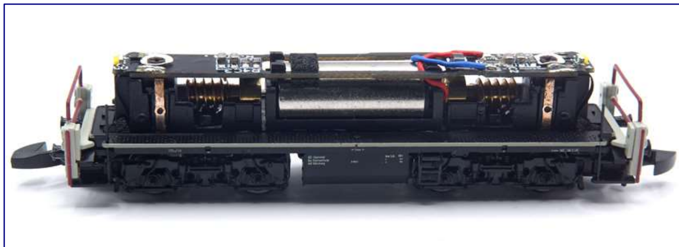
The chassis is made of plastic, which explains the remarkably low weight of this shunting locomotive. As usual, the drive works via a worm gear and spur gear.
