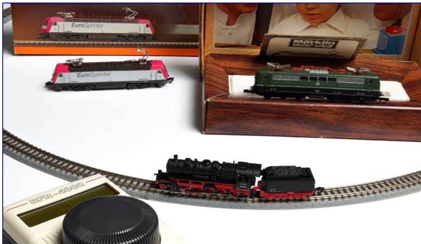
We used three locomotives with different generations of three- and five-pole motors for the test, as they require very different control systems to run smoothly.
