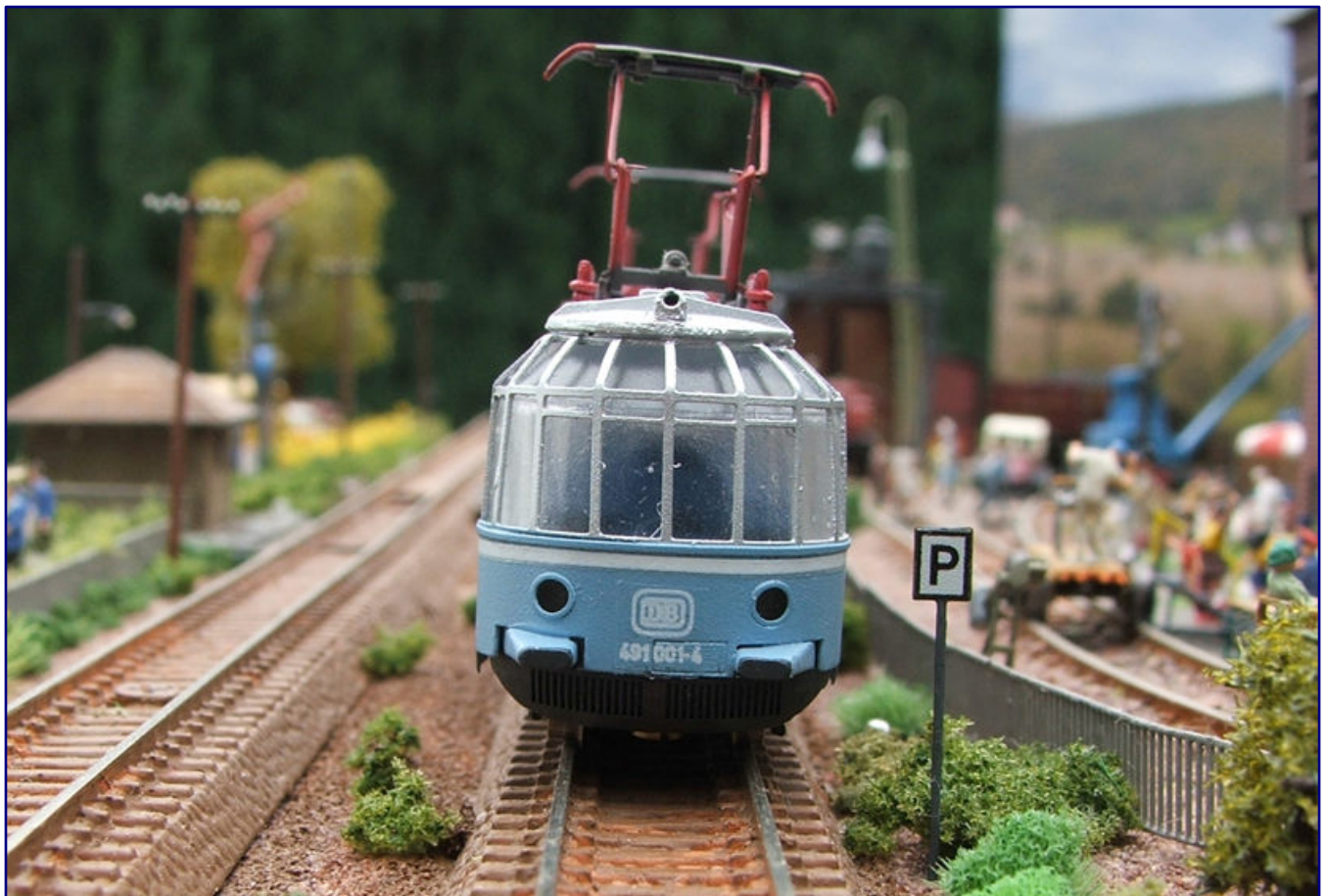
A look at the front shows some striking details of 491 001-4: Bahls Modelleisenbahnen has correctly implemented important prototypical features with the ventilator grilles below the buffers and the laterally offset maintenance access hatch between them.
