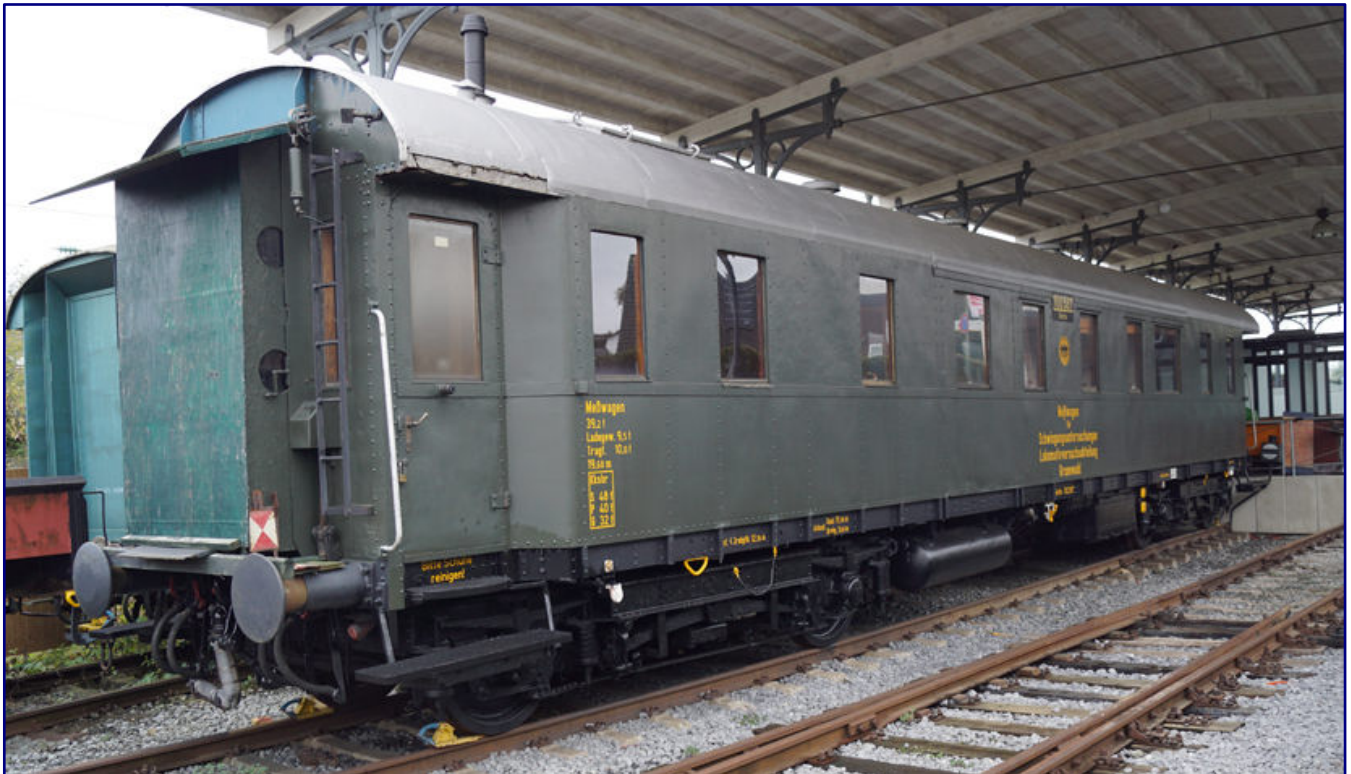
The former 700 587 Berlin measuring wagon for vibration tests at the Grunewald Research Centre was restored by the EHEH to its original appearance at the Deutsche Reichsbahn-Gesellschaft. Wolfgang Diener duplicated the historical vehicle lettering.
