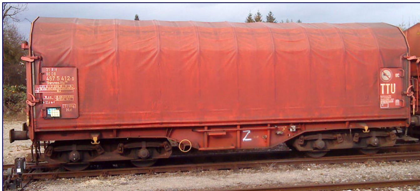
The Shimmns-ttu 722 can be recognized as a conversion wagon by its almost completely visible solebar as well as the shape of the fish belly (see photo on page 5 above). Photo: Ketamin (CC-BY-SA-3.0)
