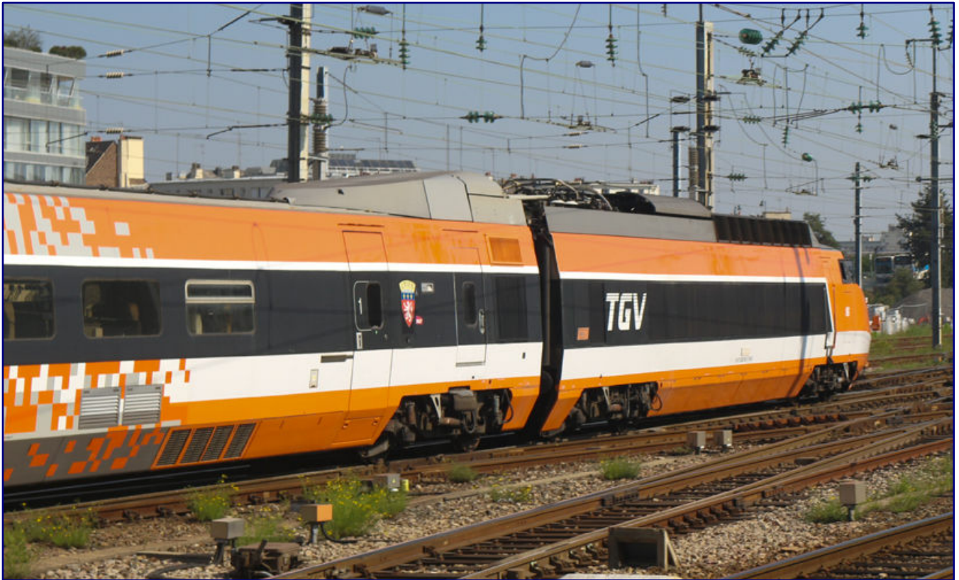
A TGV Sud Est is showcased at the Rennes station on 19 September 2024 as part of Open Monument Day. Attention is drawn to the three powered bogies of the power car and first centre carriage. Photo: Kapamez (CC-BY-SA-4.0)
