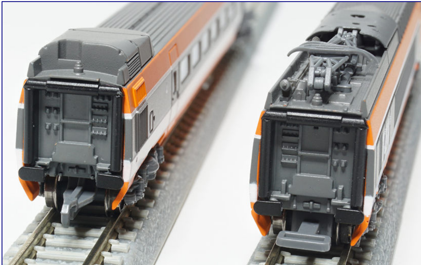
Between the motor car (right) and the end car of the articulated train (left), we find a prototypical reproduction of rubber bulges, rectangular buffers and a hint of a screw coupling.
