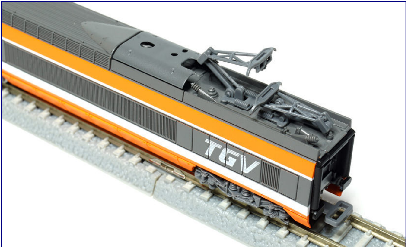
The single-arm pantographs were redesigned for the TGV, but are also to be used on other models in the future. This is probably why Azar Models opted for the DC version, even though the two models looked different in the prototype.
