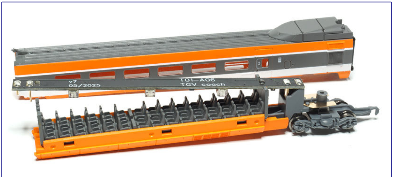
The removed housing allows a view of the interior, which features a number of details. The lighting board with its three light-emitting diodes is powered by the bogies.
