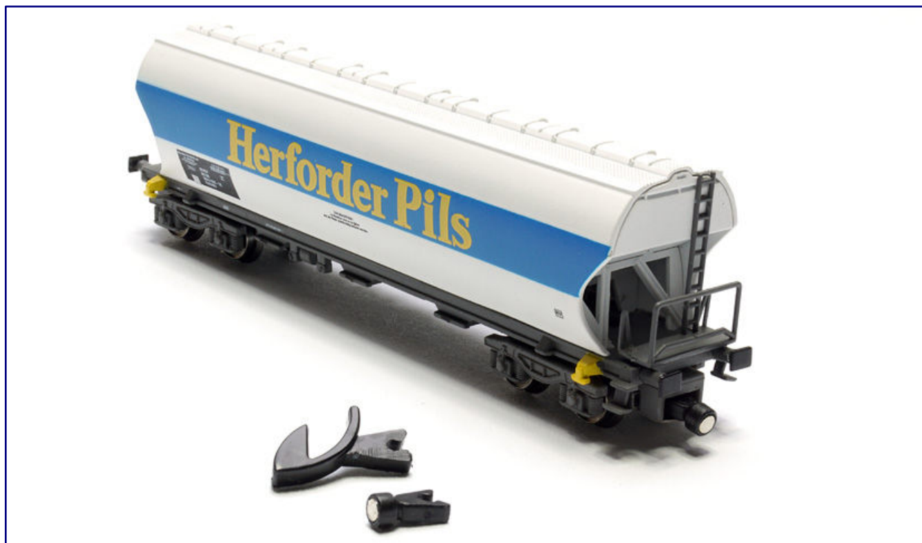
A new design is the grain silo wagon with the inscription "HerforderPils" (item no. W01-HP), which also introduces the new and significantly shorter Magnetiz coupling (shown in the picture).
