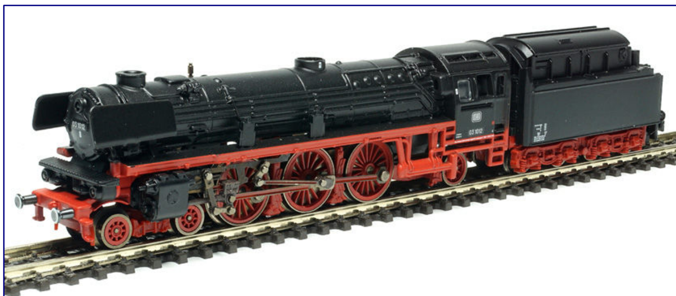
The 03 1012, fitted with a new boiler (88858), now takes on the familiar form of a steam express locomotive with spoked wheels on the leading bogie.
