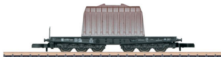
82342 - German Federal Railroad (DB) type SSym 46 heavy-duty flat car. Insulated hood for transporting hot steel. Era III.
