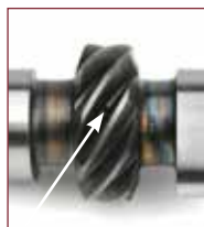
Pressure fed oiling to distributor drive gear
